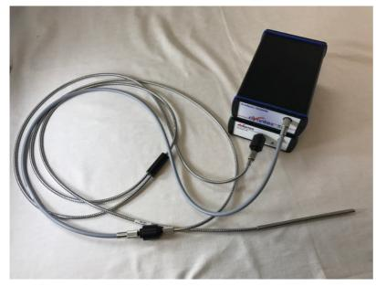
Figure 4. Typical set-up fluorescence probe configuration.
