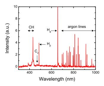
**Figure 1:** Spectrum during etching of an *a*-C:H sample, acquired with 1.3 nm resolution, 1 s integration time and averaged over 10 scans.  $H_{\alpha}$  is in saturation.
