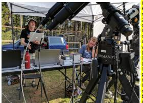
In one experiment, the HAO team used the new AvaSpec-NIR512-2.5-HSC-EVO to capture the NIR spectra from the entire corona out to 10 solar radii. In another, dual channels will collect NIR AvaSpec-NIR256-1.7-JSB2) and Visible AvaSpec-ULS2048Cl USB2) spectra from paired telescopes to take spectra of the layers of the sun's chromospere- the area between the
