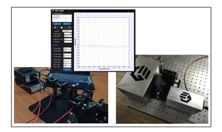
AvaSpec and AvaLight have been used to get highly accurate and stable spectra in real time speed. Thanks to the stability of these components we were able to achieve the  $\Delta(k)$  measurement repeatability of around 0.1° with the measurement speed of 20Hz. To our knowledge, this is the first dynamic  $\Delta(k)$  measurement demonstration in the spectro-polarimetry and ellipsometry.
