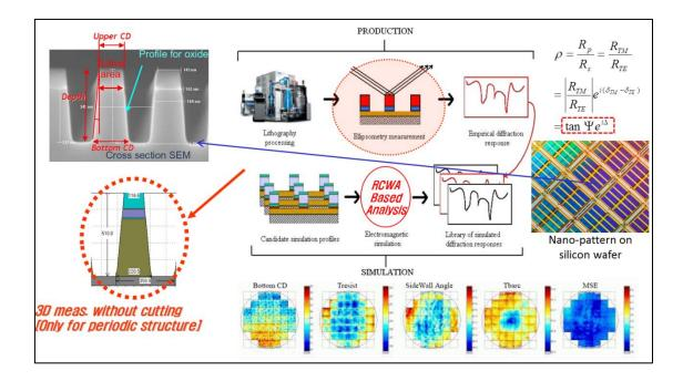
This new dynamic polarization-sensitive phase measurement technology can also be applied for in-line monitoring of transmissive anisotropic objects such as Quarter Wave Plate (QWP) or flexible nano-pattern films for Wire Grid Polarizer(WGP) etc. as illustrated below.
